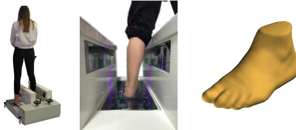
Laser digitiser for 3D capture. Source: INESCOP
