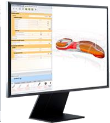
ICAD3DP, an INESCOP sole design plugin for Rhinoceros. Source: INESCOP
