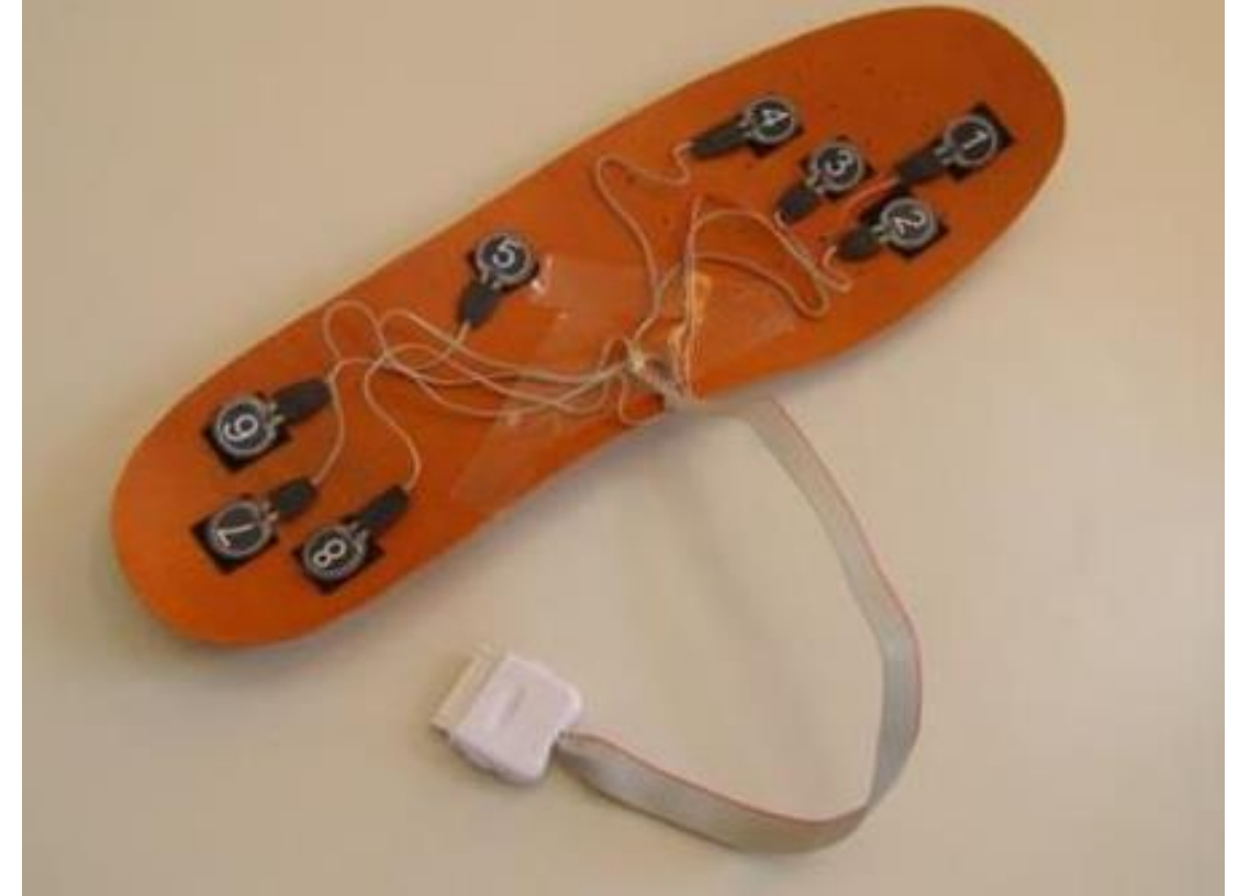
Plantar pressure distribution measurement device. Source: SCILED 2019
