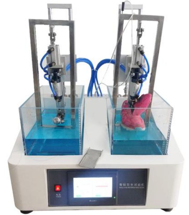
Water resistance test https://s1.amade-tech.com/wp-content/uploads/2021/02/Dynamic-Footwear-Water-Resistance-Tester-.jpg
